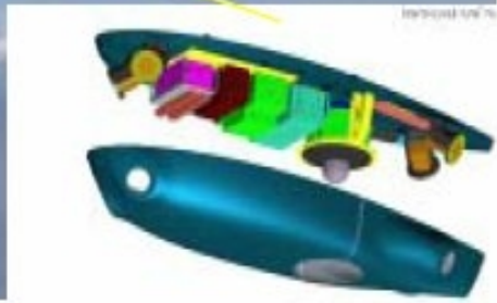
Pod with IRCM Equipment Set
